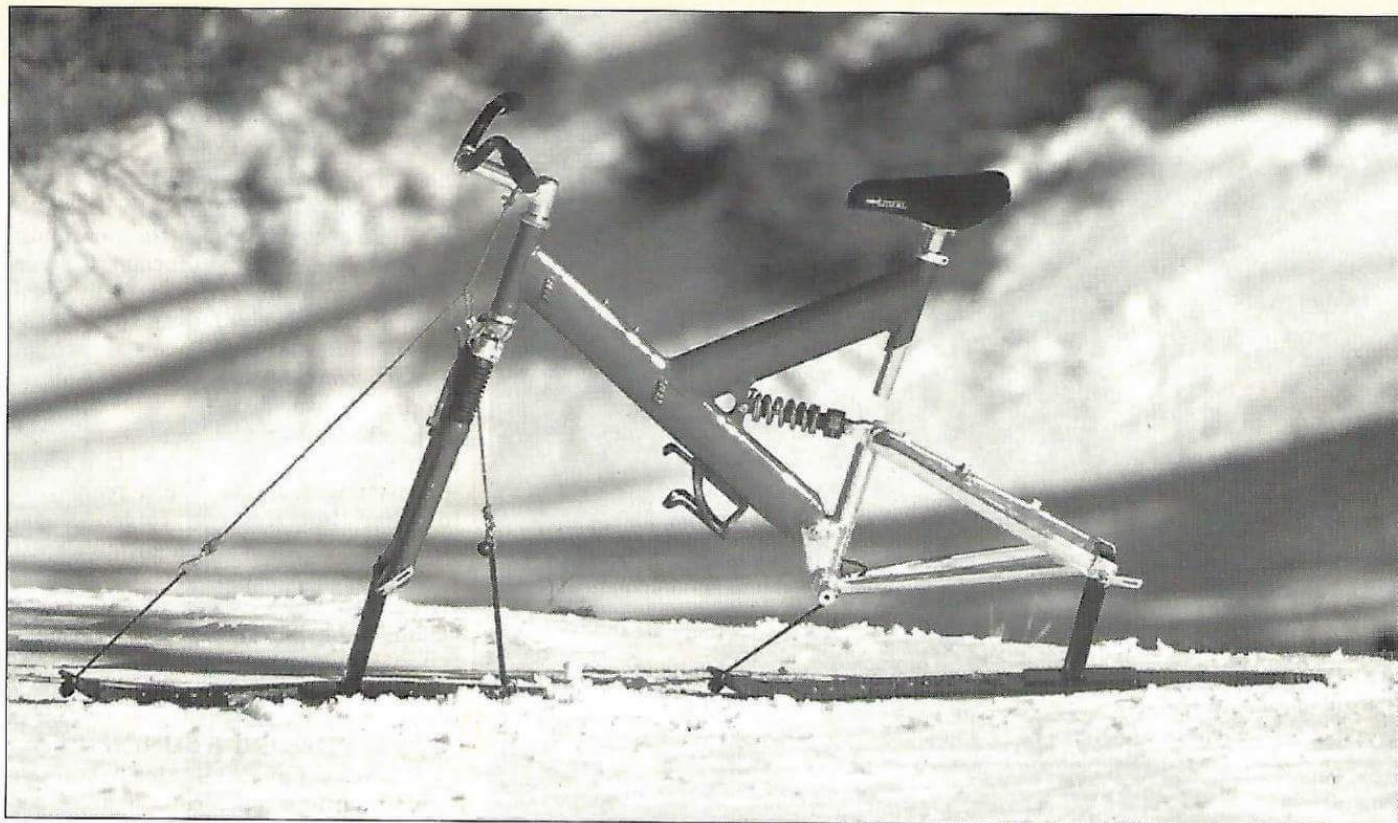
No climber: Flat Tire's Ski Bike conversion lowers the bike by about 6" and slices 2 lb. off the rolling (gliding) weight. Bungee cords hooked to the front and rear runners control ski attitude when the bike leaves the ground.
