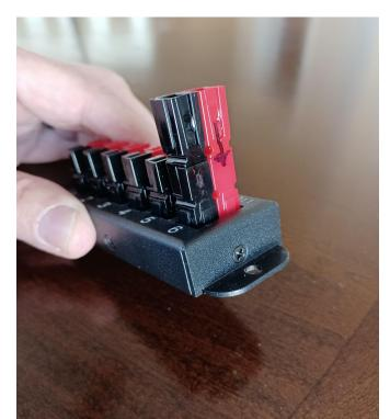
For ham radio and most other applications, the position of the two connectors is very important. This position requires that the PLUS 12 volts be on the right side (red) of the connector when looking INTO the "A", active end.
