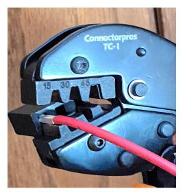
The wire going into the end of this 15 AMP size connector was stripped back 3/8 of an inch.
