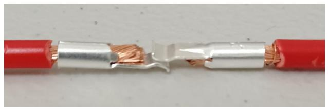
When plugging one AP into another, several problems can occur if the stripping of the wires exceeds <sup>3</sup>/<sub>8</sub> of an inch. On the left side, note the length of the center-conductor places it very close to interfering with the CONTACT POINTS between the two connectors.
