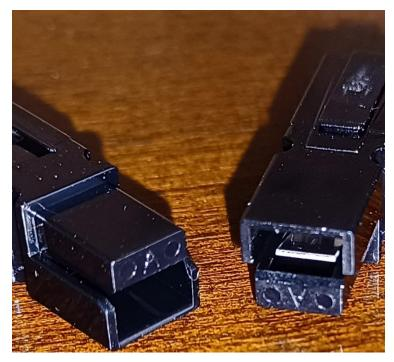
As an example, the embossed "A"s on these two black APs are shown positioned so that either one can be inserted into the other. The "A"s on each AP are in the opposite position so the two connectors can be plugged into one another.
