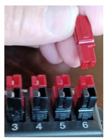
To be sure you have each pair of APs correctly positioned, take an empty pair and insert them into the target terminal strip or cable as you begin your project.
