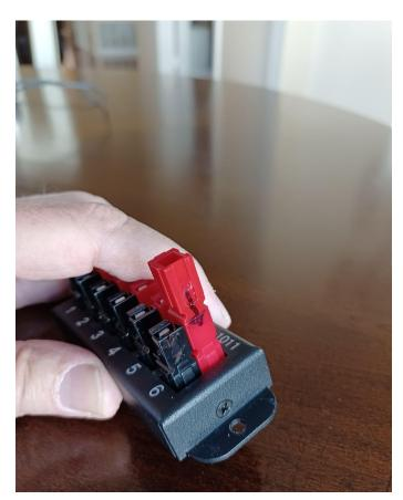
Once inserted, each Red and Black plastic piece can be marked so all the parts can be removed and later reassembled into the same position.
