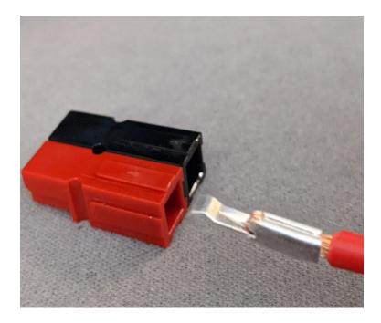
The electrical Connector, which is now crimped on a Red Wire, is ready to be inserted into a Red shell. Be sure the shell is positioned with the embossed "A" upright on the front and the Connector is flat relative to the shell before it is inserted. Repeat this same procedure with the black wire and its electrical connector as well.
