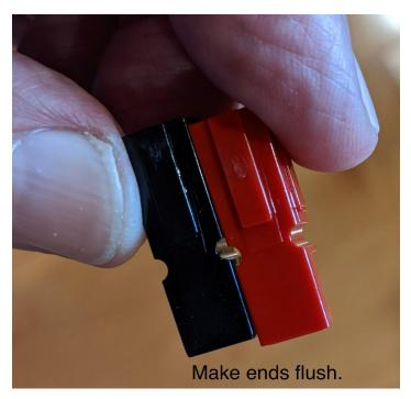
With the shells properly positioned, slide the two shells together until the "A" active ends are FLUSH on the end so the electrical connections will be solid. Because of the tight fit, you may need to gently **tap the back ends** until the front ends are flush.
