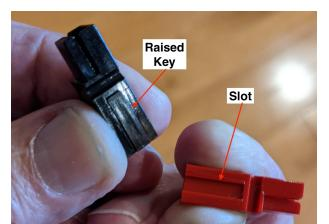
Once the correct position is determined, mate the Red and Black shells together using the slots on their sides. Here you see the flat sides on each of the shells. The raised Key on the side of the Black shell is designed to slide into the Slot on the side of the Red shell.
