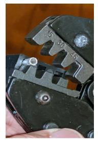
This Crimp Wrench has slots marked for each of the three-sized electrical connectors. The tongue is placed into the Crimp Wrench with the curved end facing down. Once the curved end is properly positioned within the wrench, partially compress the wrench to keep the connector from rotating while the appropriate wire gauge and length of center-conductor are inserted into the barrel for crimping.
