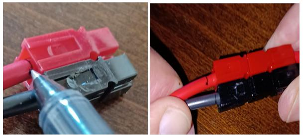
To safely disassemble an AP connector when no power is applied, gently place a small tool like a jeweler screwdriver into the back or front of the Shell to release the Capture Spring from the end of the Connector. If necessary, replace the shell or re-clamp the wires to make sure everything is totally secure in your Anderson connections. Be careful not to bend any of the metal components or it may be necessary to replace them.
