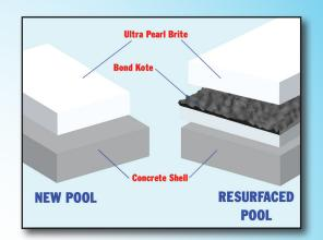
Unlike traditional pool plasters which have a history of discoloration, delamination and etching... Ultra Pearl Brite's unique formulation of the whitest marble aggregates, premium white Portland cement and performance enhancing admixtures provides the strongest and whitest marble finish in the industry. Ultra Pearl Brite's premium marble aggregates provides years of beauty and enjoyment.
