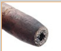
Nozzle fully clogged (not using E-Weld Nozzle)
