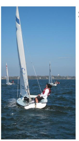
This boat is sailing in low gear. His main is slightly eased, the upper leech twisted open. He sails with a slight heel to balance the helm- which is perfect with the tiller straight down the centerline.
