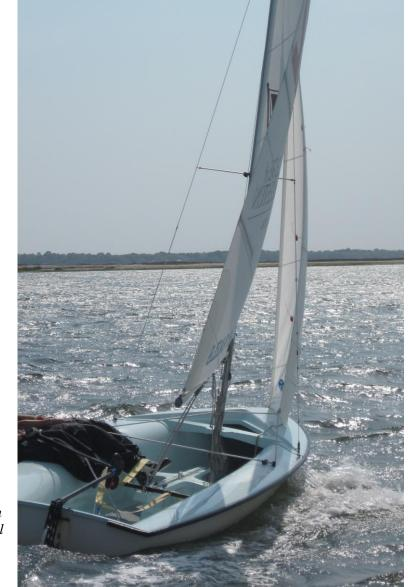
To the right is a shot showing a slightly over trimmed jib in big breeze. The slot is closed up top (no longer symmetrical with the main) and the leech telltale stalled.
