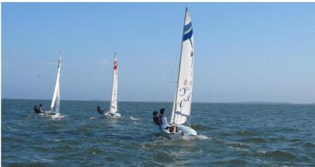
To the right, great vang tension is set for downwind sailing. The last 12-18" are almost parallel to the boom
