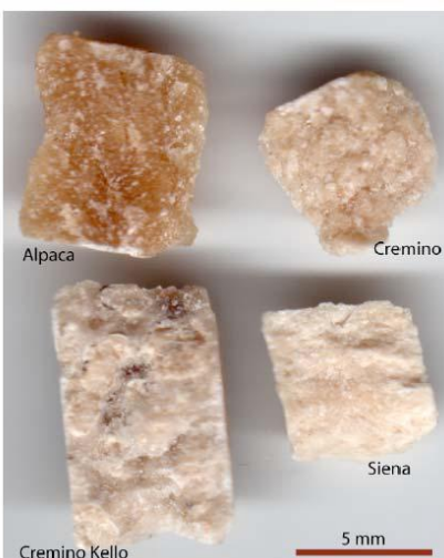
Figure 5: Fractured surfaces of the travertines, showing differences in texture and grain size. The Alpaca is relatively coarse, transparent tan calcite. The Cremino and Kello are both fine-grained buff calcite, but the Kello has a granular, “cottage cheese-like” texture whereas the Cremino has a more uniform texture. The Siena is very fine-grained beige calcite with a slightly fibrous texture (visible in the lower right portion of the chip) and uniform color. Scanned image.
