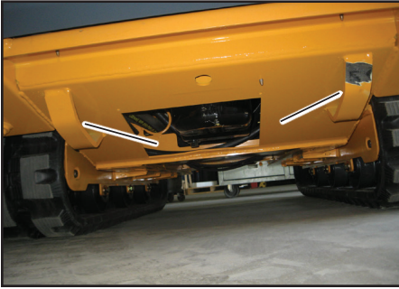
Fig. 54 - Rear Tie Down / Retrieval Points
