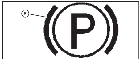
Fig. 19 - Parking Brake Button
