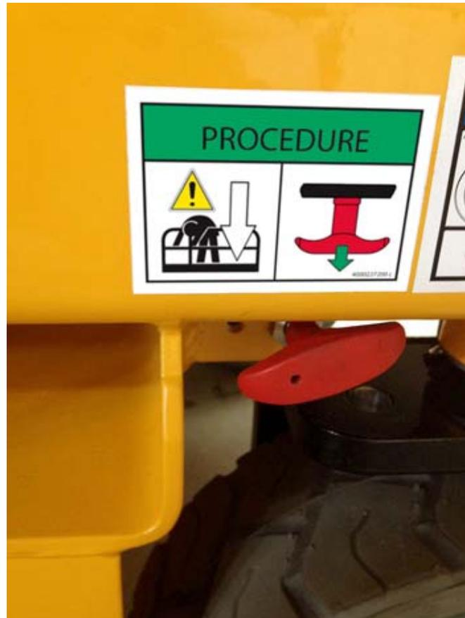
***N.B.:-PULLING ON TO THE T-HANDLE, IMMEDIATELY ACTIVATES THE EMERGENCY LOWERING OF THE PLATFORM.***
