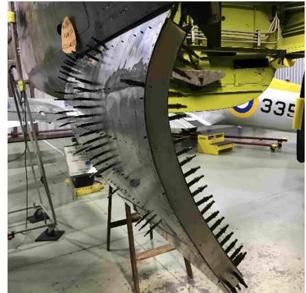
Completed door prior to disassembling
