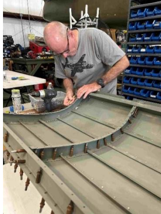
Working on stringers
