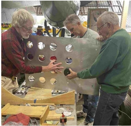
Cutting the holes in the inner skin
