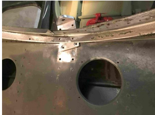
Metal bracket cleaned and ready to reattach
