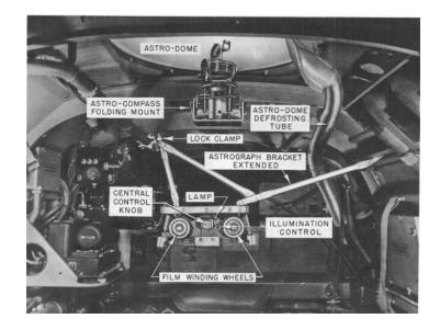
The picture above from the B-25C & D maintenance manual shows the navigator's area along with the astro-compass and astrograph. This picture is looking from the cockpit towards the back of the plane. You can see how the astrograph bracket is extended from the left side of the plane and the locking clamp attaches to the railing on the right side of the plane. Hopefully one day we will be able to restore these two instruments into GF2.
