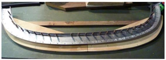
This next picture is the back wall of the bomb bay section. The vertical lines are stiffeners to strengthen the metal wall. This area has been cleaned of damaged sheet metal. The back wall will come straight down from the cross piece and attach to the curved rib pictured above. Come see this in person to understand how it will look!
