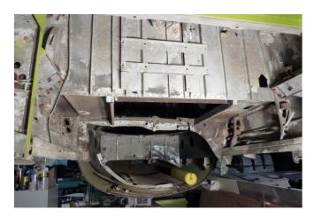
Ron has been working on the Norden bomb sight support. This is an original WWII support stand. Since the front of the plane curves up, He had to build the floor piece to make the stand sit level. The rod to hold the top of the stand level is missing. Ron has fabricated a new piece from scratch. Even the latch and thumb lever are hand-made! The detail in this piece needs to be see in person to be truly appreciated!
