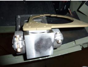
Note the hand-made thumb lever and latch
