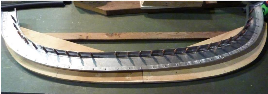
This next picture is the back wall of the bomb bay section. The vertical lines are stiffeners to strengthen the metal wall. This area has been cleaned of damaged sheet metal. The back wall will come straight down from the cross piece and attach to the curved rib pictured above. Come see this in person to understand how it will look!
