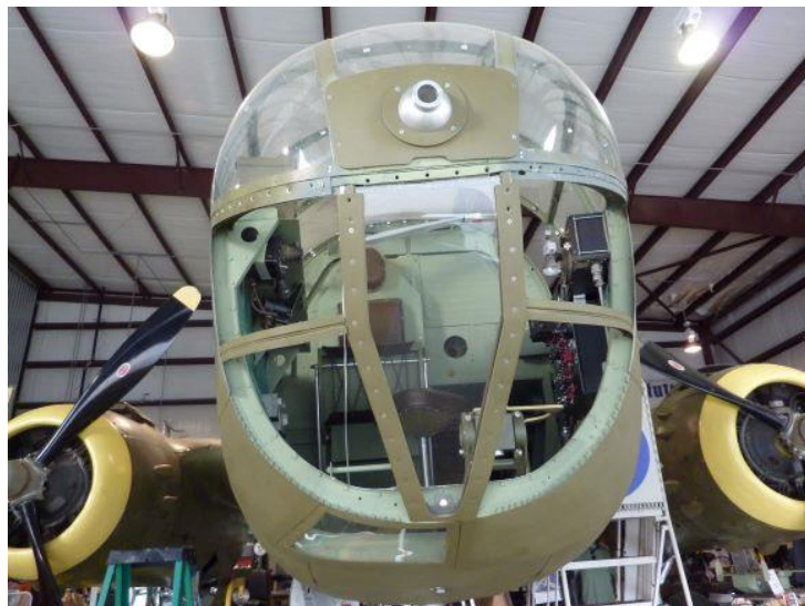
Nose pieces installed
