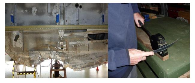
We are not sure if some of the damage to the bottom of the fuselage was a result of the crash or a result of raising the plane from Lake Greenwood. In order to make the needed repairs around the bomb bay doors, we are making a new piece for the bottom
