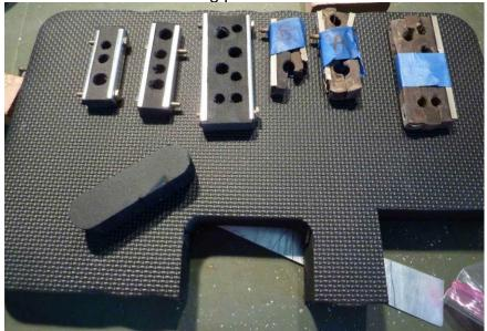
This picture shows three of the gas transfer valves we removed from the bomb bay section. These will be cleaned and reinserted into the plane. There are a couple of original hoses still in the plane that will be reattached. We will then find new hoses to fill in the rest of the area.
