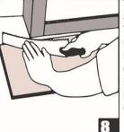
The gap between the bottom of a door and the vinyl flooring should be 1 cm height. To trim door frames, turn a plank upside down. Place it next to the door frame as per diagram.
