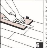
To fit the final row, lay a plank upside down on the flooring as per diagram with the tongue side close to the wall. Take another plank and place it right on top of the previous row and use it as a ruler. Don't forget to allow room for spacers. Cut the plank and attach into position.
