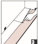
For the last plank of a row, flip a full plank to its under side and place beside the row. Measure and mark the required length.
