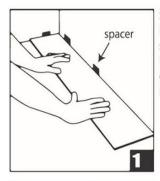
Start at a corner. Place first plank with tongue side facing wall. Use spacers to maintain an expansion space of 2-3 mm between wall and flooring.
