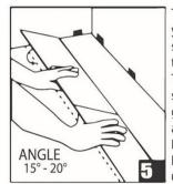
To start second row, assemble your entire row on the subfloor before attaching it to the first row. To attach, tilt and push the side tongue into the side groove of the first row at an angle of 15° to 20°. Lower and click into place lining the edges up carefully. Continue laying remaining planks in this matter.
