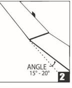
Insert 2nd plank's end tongue to 1st plank's end groove at an angle of 15° to 20°. The plank will click into place when lowered. Line up edges carefully. Planks should be flat to the floor.
