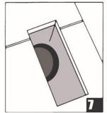
Heating vents require expansion room. First, cut plank to the correct length. Place the cut plank at its actual position and use a ruler to measure the areas to be cut out and mark them. Cut out the marked points allowing the neccessary expansion distance.
