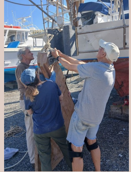
Volunteers including, from left, Dave Croy, Dana Briggs and Steve Heare, stabilize the 250-pound rudder as it is suspended for applying epoxy. Photo by Tina McCloud
