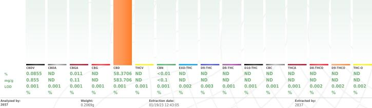
Analysis Method: SOP.T.30.031.TN & SOP.T.40.031.TN Expanded Measurement of Uncertainty: Flower Matrix d9-THC: ± 0.100, THCa: ± 0.124, TOTAL THC ± 0.112. These uncertainties represent an expanded uncertainty expressed at approximately the 95% confidence level using a coverage factor k=2 for a normal distribution.
