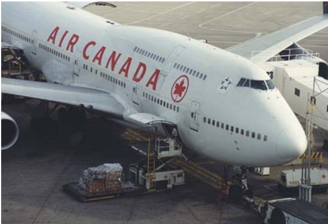
Above: Boeing 747 on ground loading cargo through opening outward nonplug forward cargo door. The tiny dot of the one midspan latch on the leading edge of the door can be seen.
