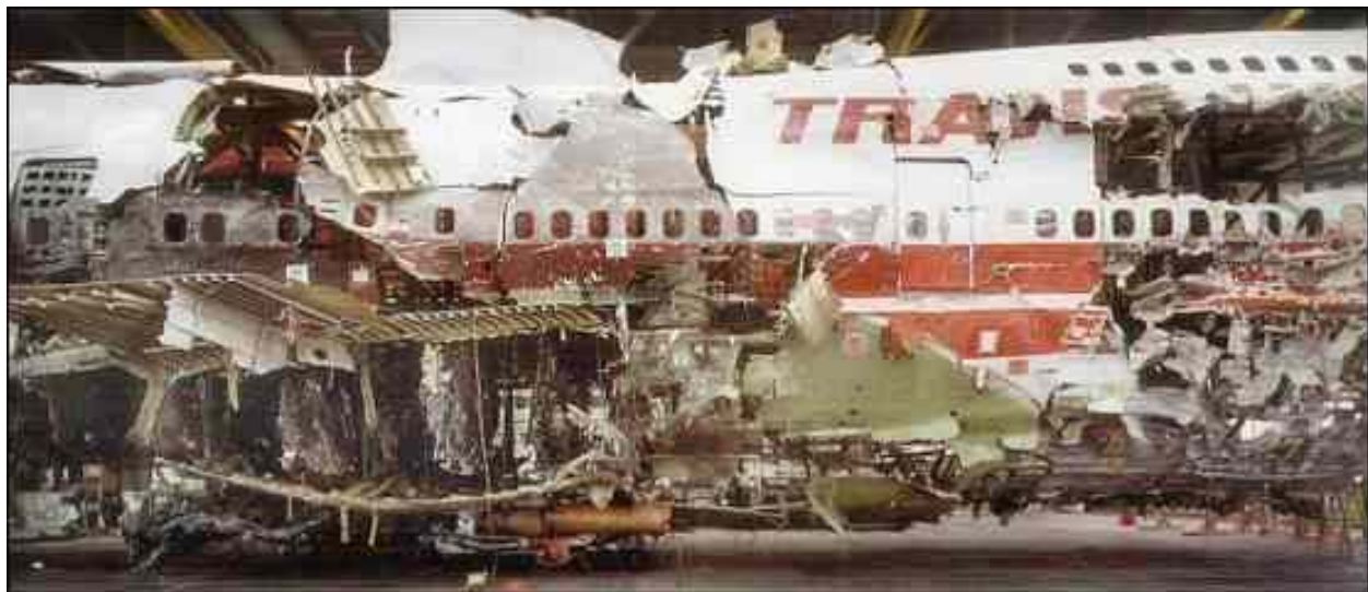
Right front and middle of Trans World Airlines Flight 800 revealing sharp sooted and non sooted cut in fuselage, nose to right.
