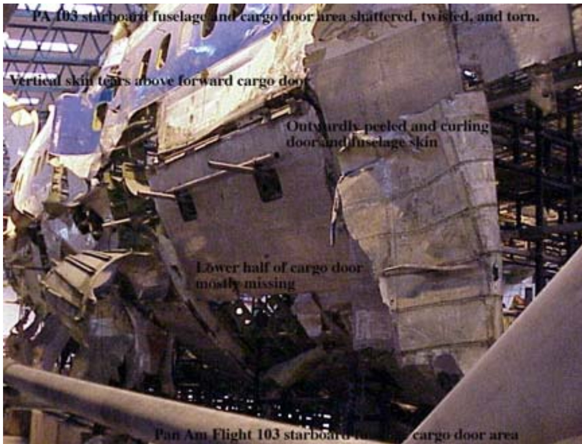
Photograph from AAIB showing Pan Am Flight 103 forward cargo door area revealing the vertical torn skin above door, peeled back and down skin from the aft midspan latch, generally shattered area, and mostly missing lower half of door which includes the manual locking handle and the eight bottom latches.
