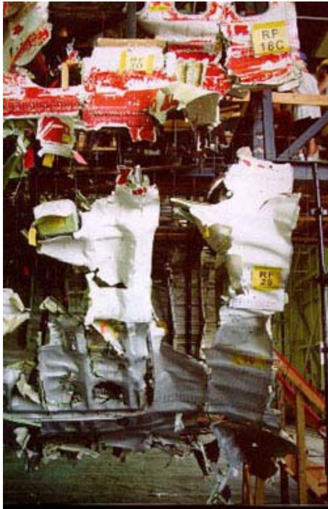
Above is a closeup photograph of about a half of the Trans World Airlines Flight 800 forward cargo door extending from fuselage station 520 on the right to fuselage station 620 to the left in the photograph. The cargo door hinge is in red near the top of the photograph. The outward opening petal shaped oval rupture is located at the forward midspan latch of the forward cargo door.
