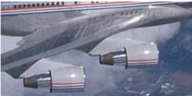
Engine number three is on the right side inboard and would be the engine to throw off a stator blade to penetrate the right horizontal stabilizer. Engine number four is too far outboard of stabilizer. The left side stabilizer had no such engine part penetration.
