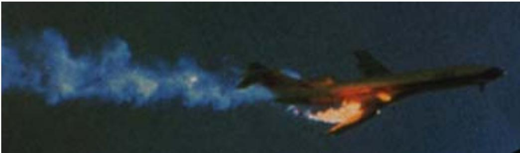
This is a Boeing 727 that had a mid-air collision. Fuel is leaking from the wing tanks and is on fire. Note there is no streak to leaking fuel on fire. Note fire stays close to aircraft. Note there is no explosion. Streak observed for TWA 800 was not leaking fuel on fire from center tank, it was shiny metal object spinning away in red-orange sunlight being perceived as streak to observers below.
