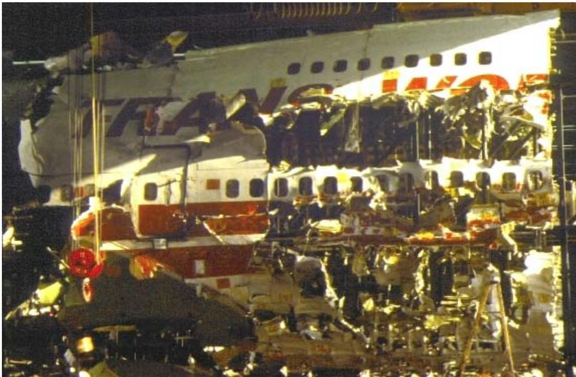
11. May, 1997, TWA 800 reconstruction of fuselage wreckage is completed. Outward bulge of door frame, red paint smears above cargo door on white fuselage, missing/not hung aft midspan latch, outward peeled upper skin, rupture hole at aft midspan latch, and larger explosive decompression shape become apparent in photograph of reconstruction.
