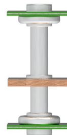
Example of power tap pin using two sockets to connect three boards/busbars
