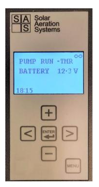
The remote control runs from 2 off AAA batteries.
