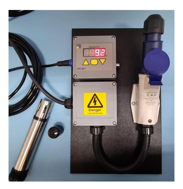
The DO5021 optical probe is supplied with 5 mtrs cable as standard but can be increased with connectors or single length at the factory.
