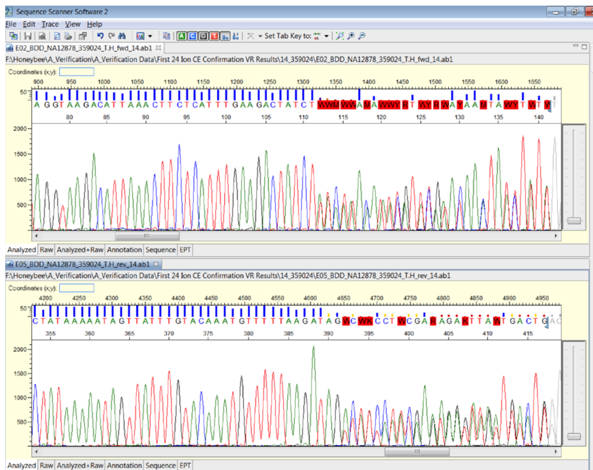
Figure 57. Sequence scanner view of a heterozygous insertion deletion (het indel). Het indel is a scenario in which one allele contains a specific insertion or deletion that the other allele lacks, putting the sequence content out of phase at the point of the particular insertion or deletion. This is a true biological event and can usually be confirmed through alignment of both forward and reverse trace files against a reference sequence to determine the insertion or deletion.
