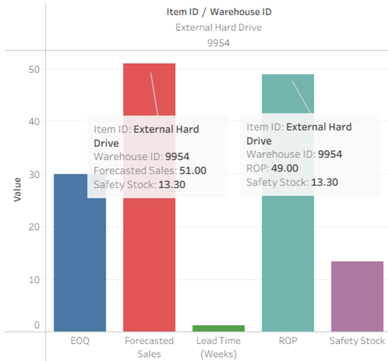
Fig: ROP based on forecasted demand during lead time, illustrating how service level (70%) impacts safety stock and consequently the overall reorder point.
