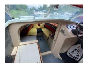
The cabin consists of a forward V berth with infill to make a double bed, then storage lockers to port and starboard with sink and space for a stove for those essential cups of tea and coffee.
