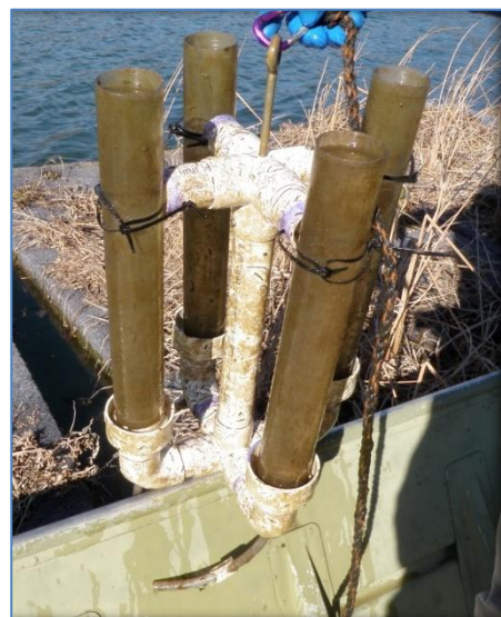
Figure 4 Sediment trap collection device.
