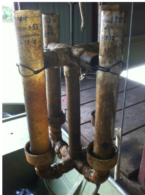
Figure 10 Sediment trap retrieved from under the floating wetlands.
