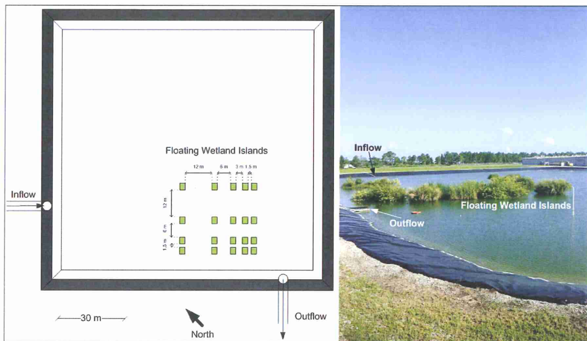
Figure 1. Placement of Floating Wetland Islands and Typical View, showing relation of islands and pond outlet.
