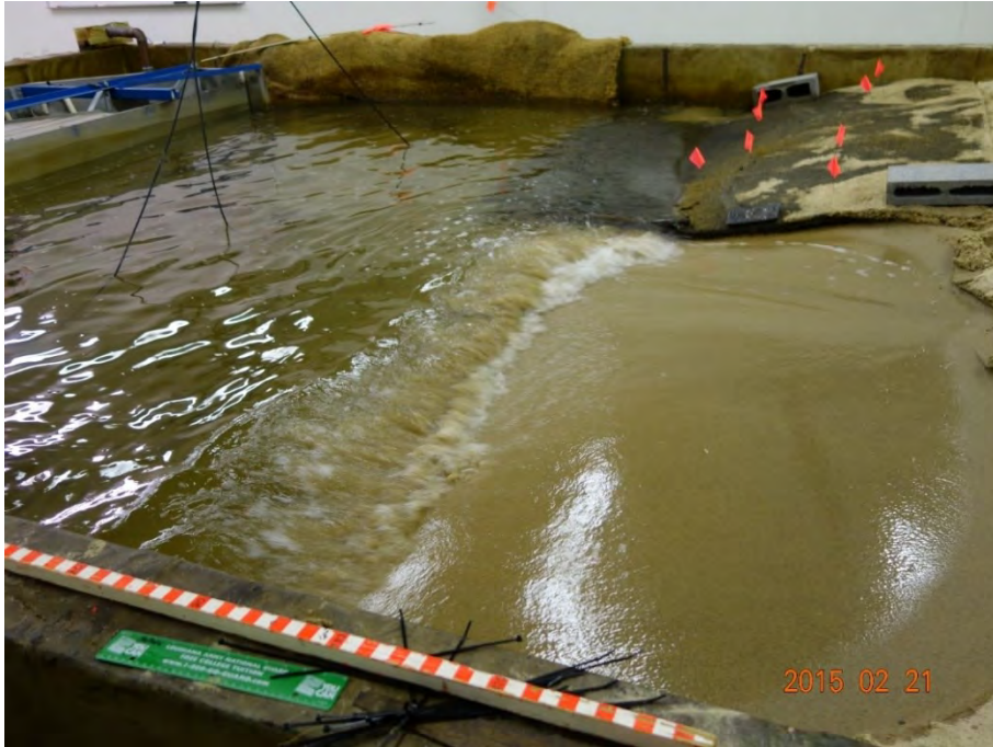
Photo 8: Showing the wave breaking in front of the bare side but wave height suppressed in front of the EcoShield™ mat.
