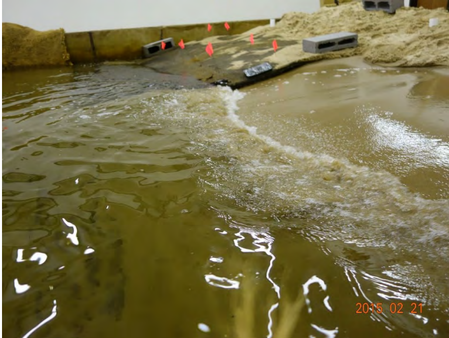
Photo 6: Showing the wave breaking in front of the bare side but wave height suppressed in front of the EcoShield™ mat.
