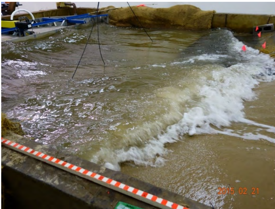
Photo 9: Showing the wave breaking in front of the bare side but wave height suppressed in front of the EcoShield™ mat.
