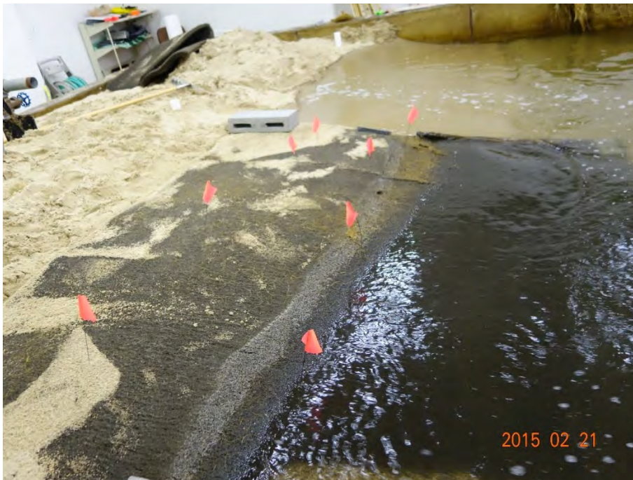
Photo 7: Showing the wave reaching further on beach in front of the bare side than that of the EcoShield™ mat.
