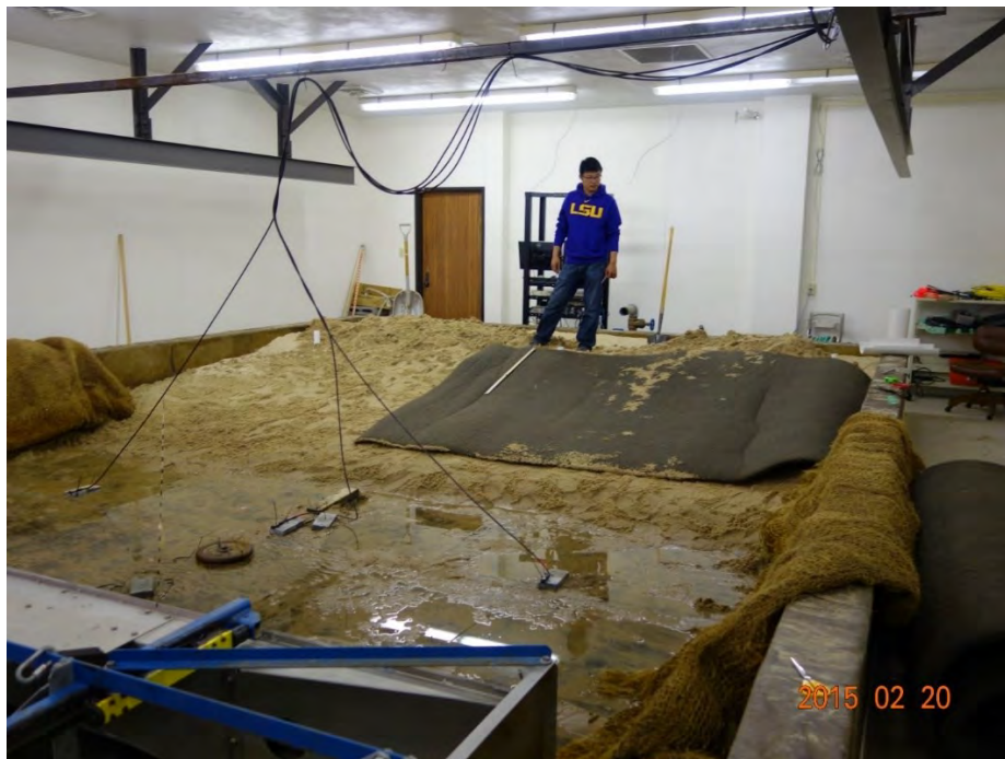
Photo 1. before cutting the mat: The sensors are numbered from left to right. The first sensor is at the end of the left most line with the pressure sensor tied to a lead weight, with a red band around the cable near the end of the cable. The second sensor tied to a lead weight is in the middle with two red
