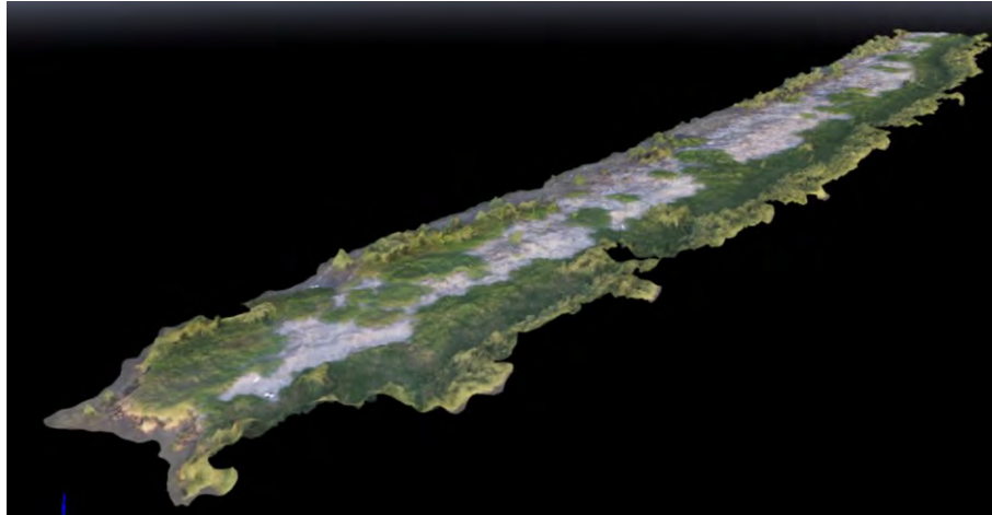
Figure 39. The DSM model of the earthen berm derived from the drone images.
