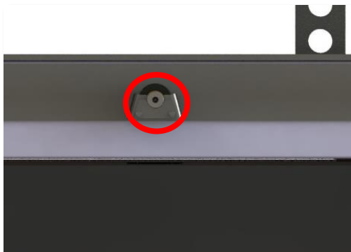
6. GREASE POINT AT SLIDING ROLLER PIN (8) (Not Applicable for IR/VAN Spec)
