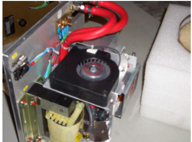
Close-up of a liquid-cooled microwave power generator.
