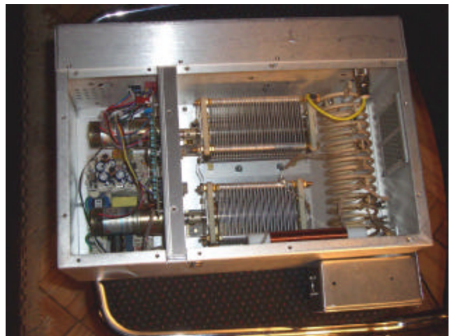
Close-up of RF matching network showing stepper motors.
