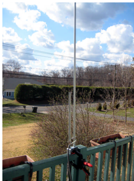
My second Queen Creek Easy J-Pole Antenna (my first lives in Arizona.) temporarily installed on my front porch.
