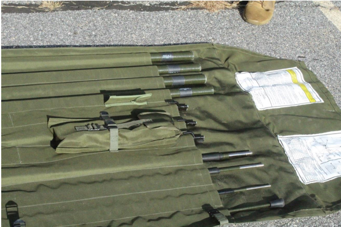
National Guard portable HF vertical antenna system
