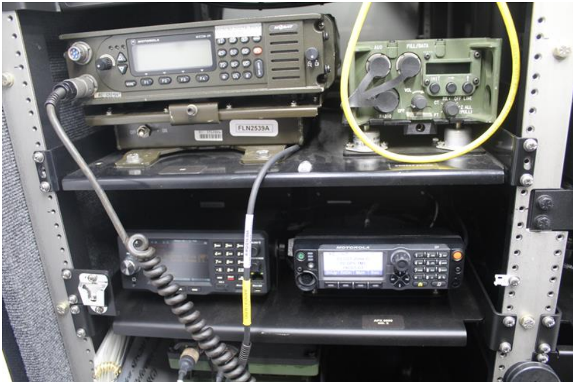
Interior rack with HF/VHF/UHF radios
