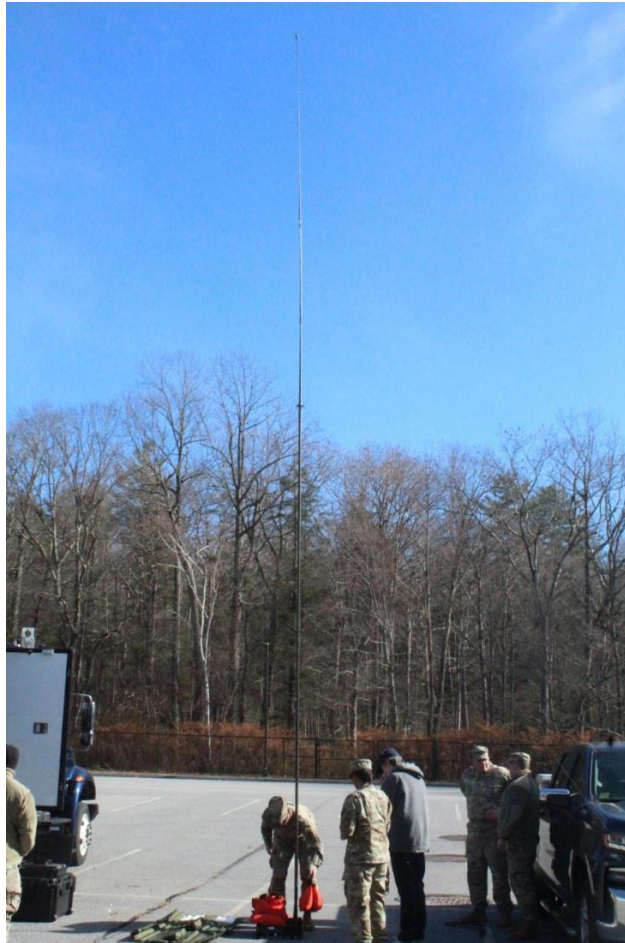
Assembled & deployed National Guard portable vertical HF antenna system
