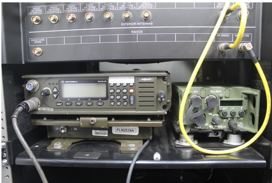
Interior rack with HF/VHF/UHF radios
