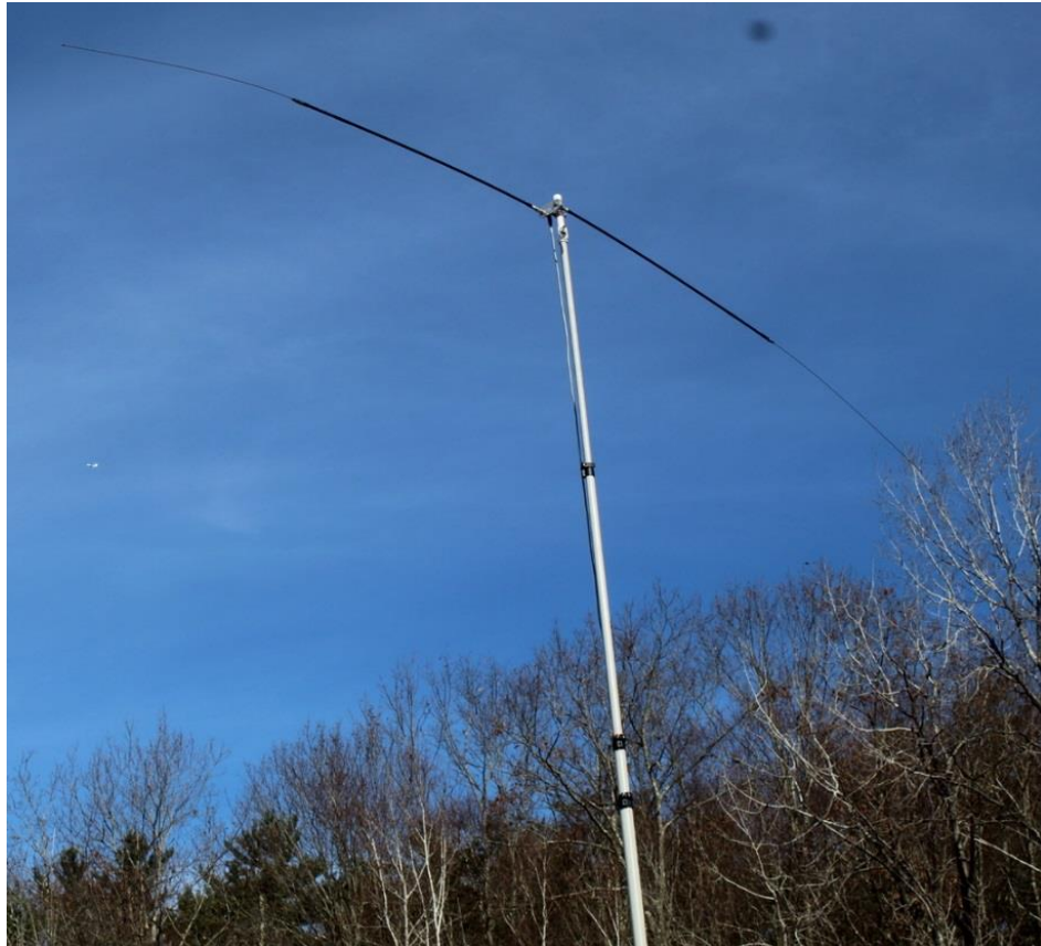
20M (14 MHz.) Ham-stick dipole on 25 Ft. portable telescoping fiberglass mast
