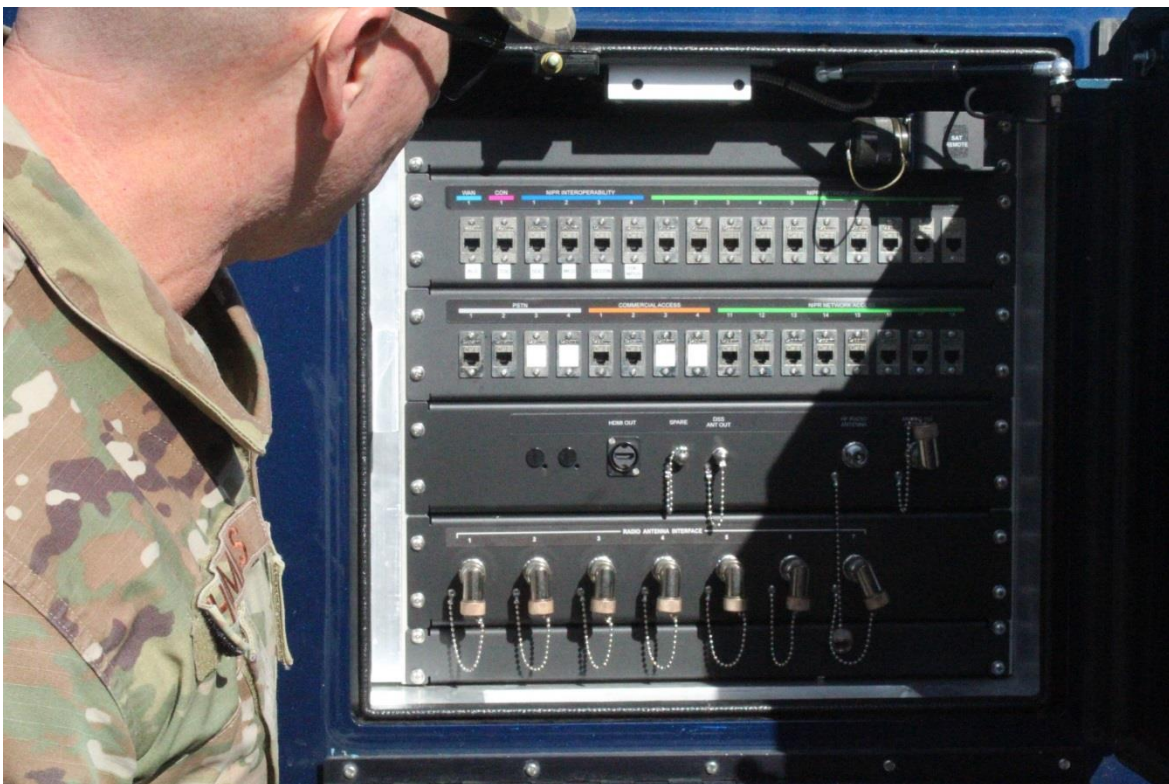
Side access panel and door for external vertical HF antenna system connections.
