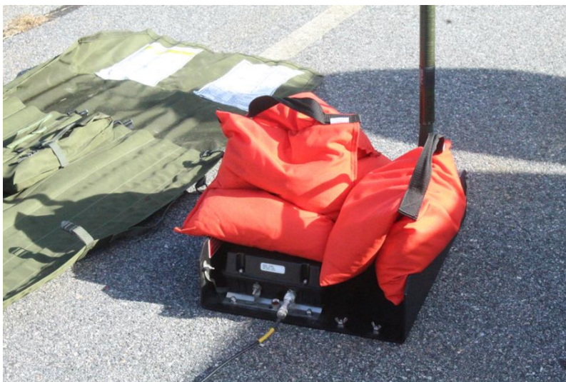
Sandbags for external portable HF vertical antenna system stability
