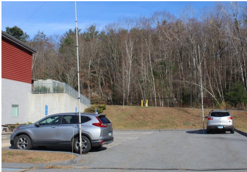
Portable telescoping fiberglass masts for Amateur Band antenna support
