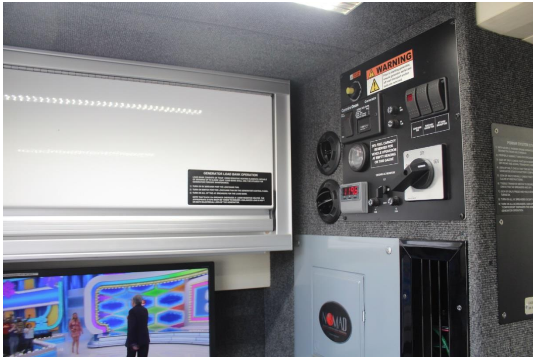
Interior equipment rack with pneumatic mast and satellite receiver controls
