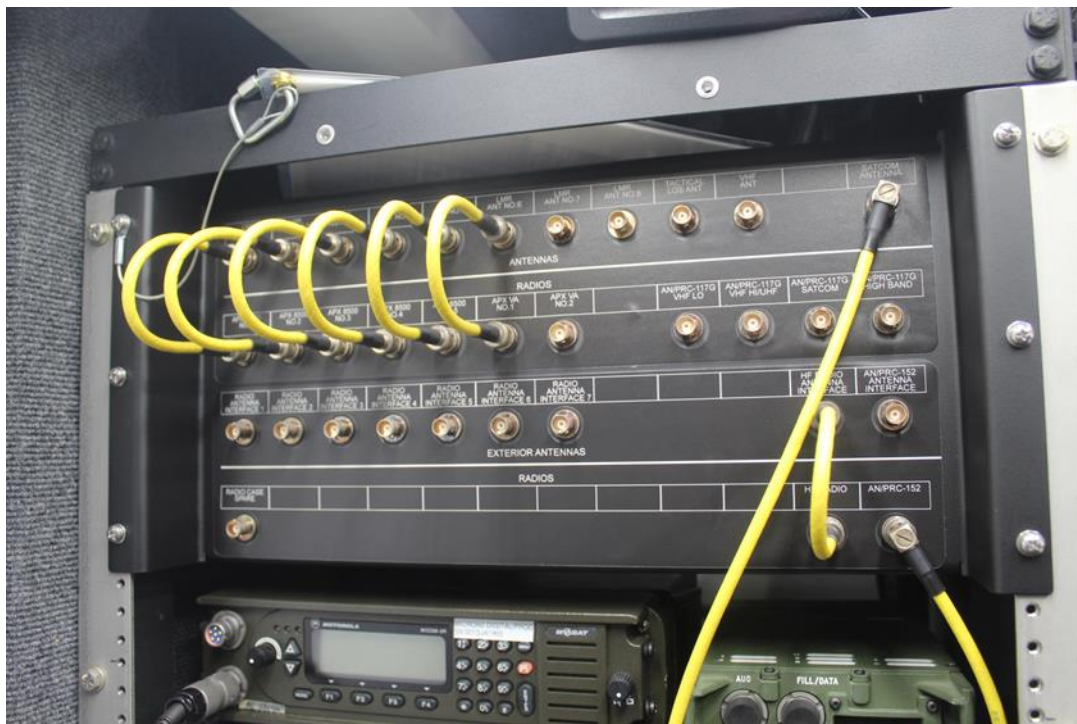
Interior rack with antenna jumper bulkhead panel
