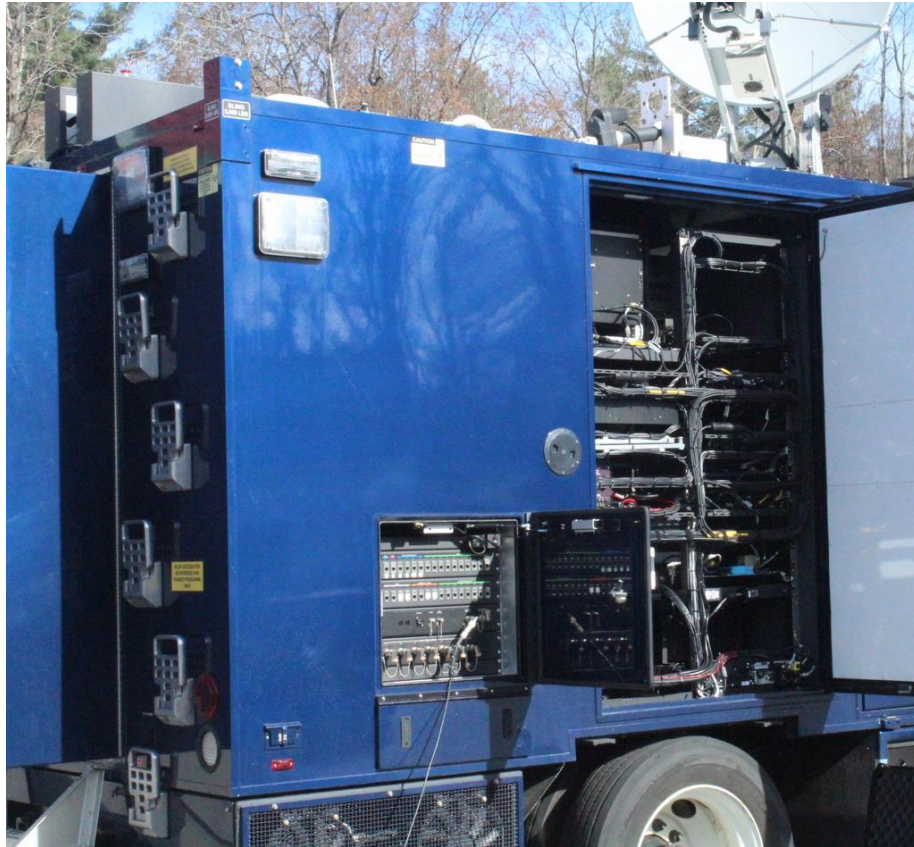
Side access panel and door for external vertical HF antenna system connections.
