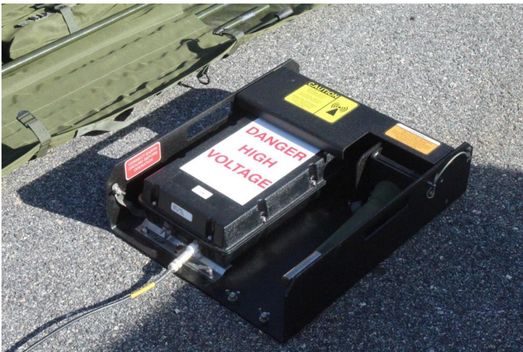
External HF vertical antenna base with built-in matching system
