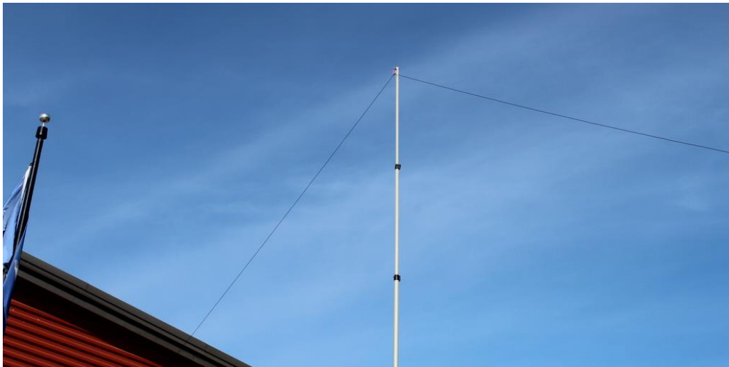
End-fed wire antenna supported by 25 Ft. portable telescoping fiberglass mast
