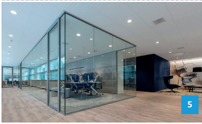
Slimline Clearvision 30 Single glass, Rw=39dB, tracks: 1.18 inches, glass to glass connection: flush-joint
