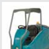
Protect operators from falling objects with the optional **overhead guard**.
