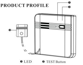
3 Sensor (Built-in magnet has adsorbed function)
