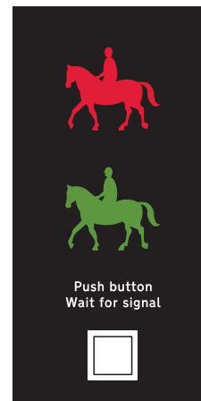
Near-side signals for equestrian crossing
