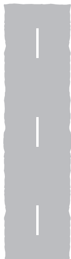
Centre line on a single carriageway road
