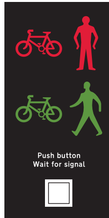
Near-side signals for Toucan crossing
