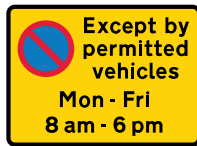
Repeater sign within a loading area
