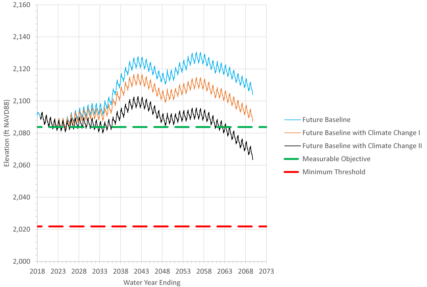
Figure 3-30. Predicted Hydraulic Heads at Hog Canyon 2 in the Calimesa Management Area
