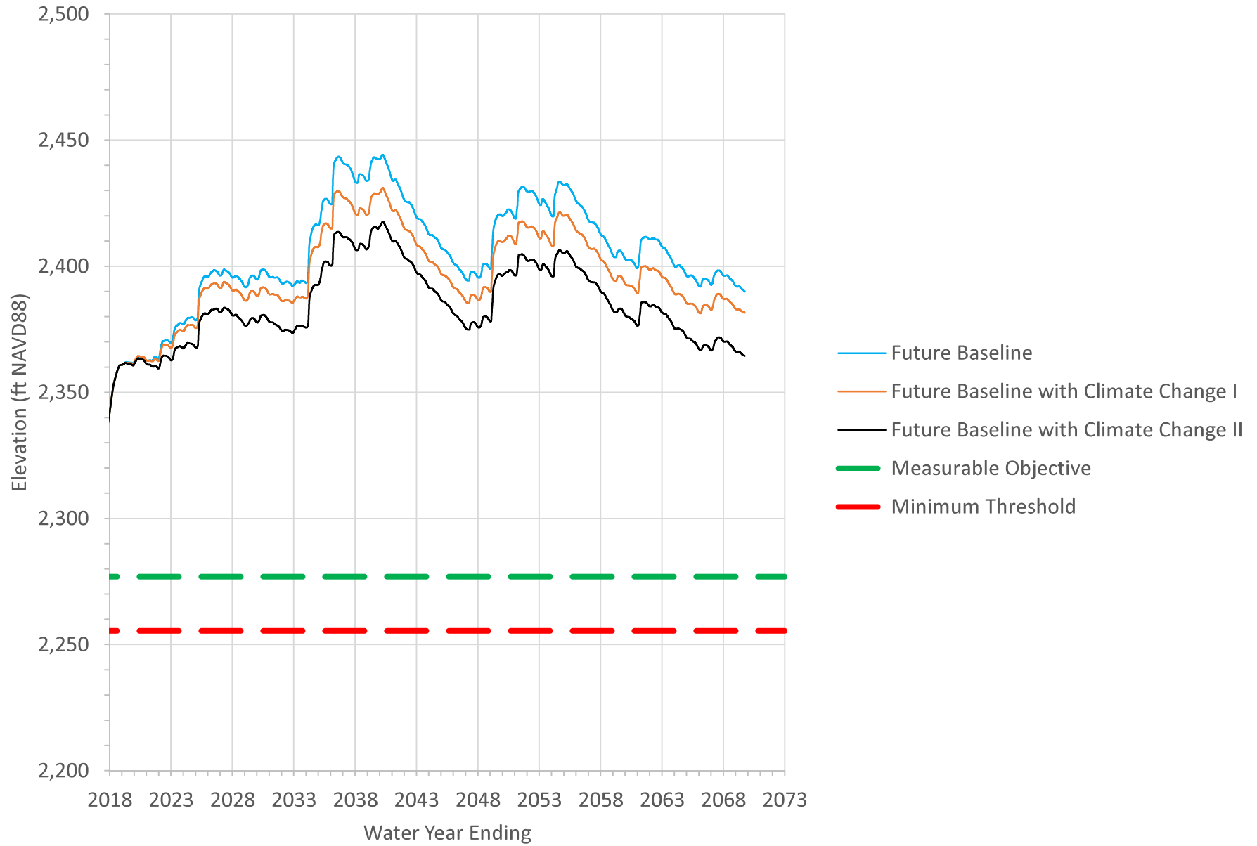
Figure 3-7. Predicted Hydraulic Heads at YVWD-06 in the North Bench Management Area
