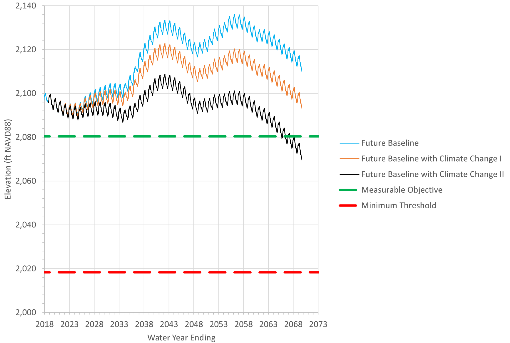
Figure 3-24. Predicted Hydraulic Heads at South Mesa 12 in the Calimesa Management Area
