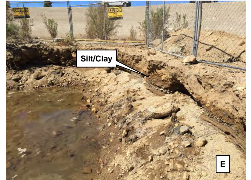
A. 4" fire hose / YVWD fire hydrant in background B. Post-excavation / fencing setup (Day 1) C. Test in progress (Day 3) D. Test in progress (Day 4) E. Post-testing - hard silt/clay layer shown in upper 3 feet
