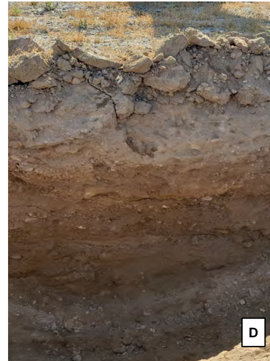
A. Initial excavation of test infiltration basin B. 4" fire hose through intra-basin culvert C. Clay on basin surface from historical SWP recharge operations; SWP water during test release from turnout D. Fine-grained silt/clay 0-2.5 feet; silt/sand/gravel 2.5-5 feet E. Test in progress (Day 11) F. Dry basin after falling-head test (Day 14)
