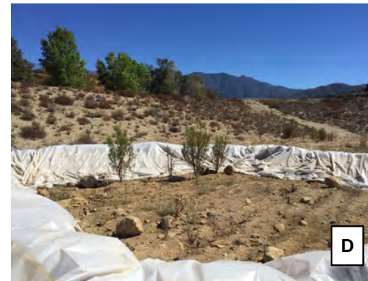
A. 4" fire hose / YVWD fire hydrant in background B. Bermed (background) and Excavated Basin (foreground) C. Fine silt/clay on ground surface D. Post-excavation and plastic sheeting bermed basin E. Testing in progress (Day 1) F. Leaked recharge water east of test basin (Day 6)
