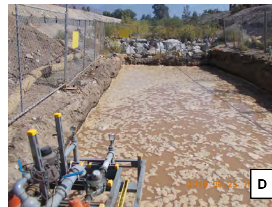
A. YVWD hydrant at 10th Street and 4" fire hose B. 4" fire hose along northern channel bank west of 10th Street C. Excavated basin, fencing, and soil stockpile D. Initial test basin filling (Day 1) E. Falling head test in progress view from south (Day 2)
