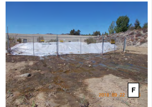
A. 4" fire hose / YVWD fire hydrant in background B. Bermed (background) and Excavated Basin (foreground) C. Fine silt/clay on ground surface D. Post-excavation and plastic sheeting bermed basin E. Testing in progress (Day 1) F. Leaked recharge water east of test basin (Day 6)
