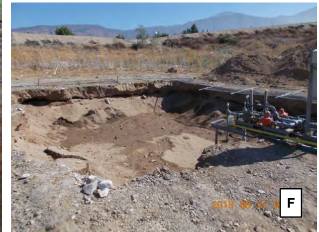
A. Initial excavation of test infiltration basin B. 4" fire hose through intra-basin culvert C. Clay on basin surface from historical SWP recharge operations; SWP water during test release from turnout D. Fine-grained silt/clay 0-2.5 feet; silt/sand/gravel 2.5-5 feet E. Test in progress (Day 11) F. Dry basin after falling-head test (Day 14)
