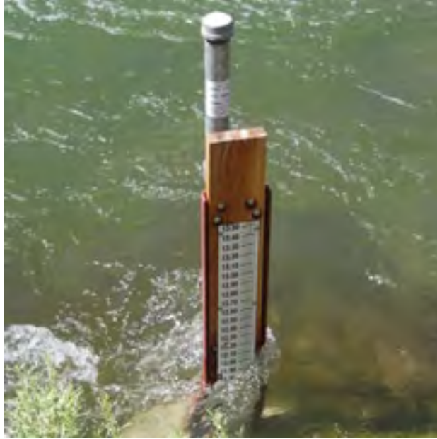
Figure 6 – Simple Stilling Well and Staff Gage Setup
