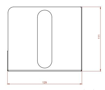
Height: 111mm Width: 129mm Depth: 129mm Weight: 0.5Kg Capacity: 250 Napkins (Approx)
