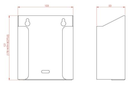
Height: 121mm Width: 103mm Depth: 53mm Weight: 0.3Kg Capacity: x1 500ml Carex Bottle
