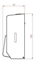
Height: 196mm Width: 96mm Depth: 97mm Weight: 1Kg Capacity: 400ml
