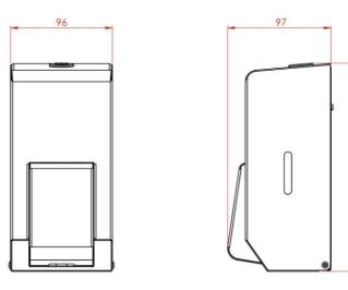
Height: 196mm Width: 96mm Depth: 97mm Weight: 1Kg Capacity: 400ml
