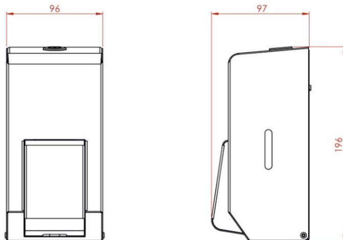
Height: 196mm   Width: 96mm   Depth: 97mm   Weight: 1Kg   Capacity: 400ml
