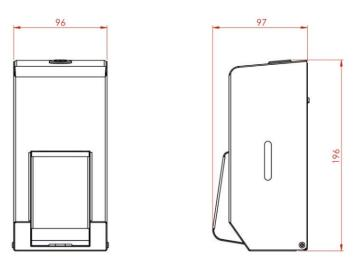
Height: 196mm Width: 96mm Depth: 97mm Weight: 1Kg Capacity: 400ml
