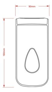
Height: 190mm Width: 90mm Depth: 98mm Capacity: 400ml
