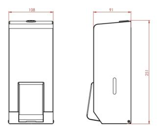
Height: 251mm Width: 108mm Depth: 91mm Weight: 1.2Kg Capacity: 900ml
